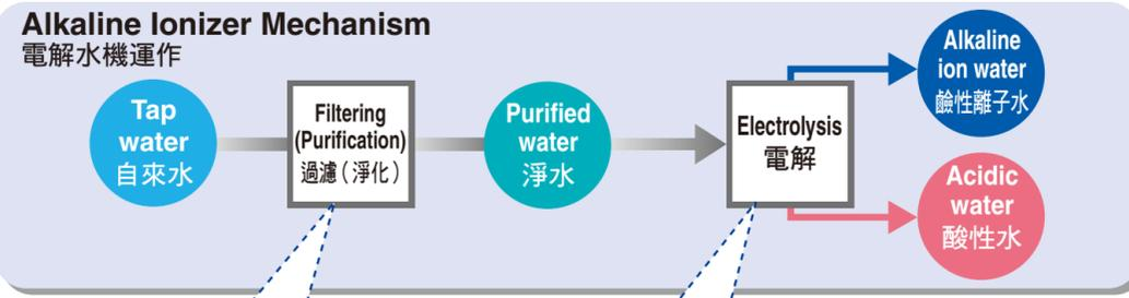
**Alkaline Ionizer Mechanism 電解水機運作**
