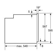
\* 20mm for metal fascias Measurements in mm
