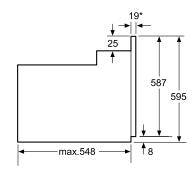
\* 20mm for metal fascias Measurements in mm
